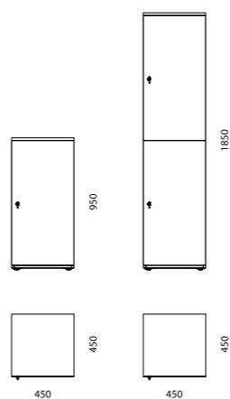
**Locker with rod (depth 600 mm)**
