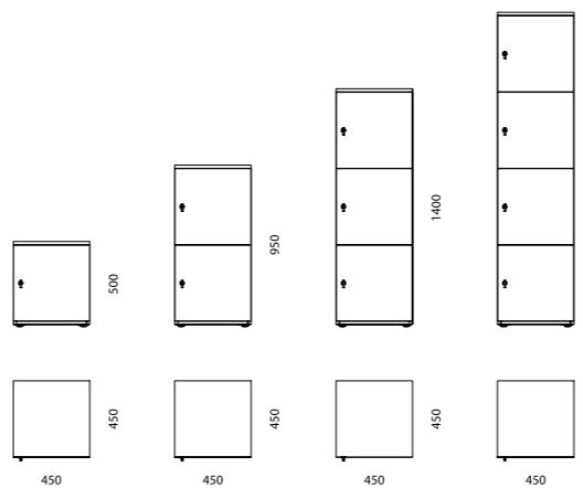
**Locker for trolley (depth 450 mm)**
